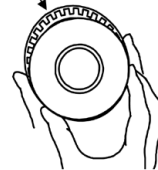
Fig. 2 Removal of the piston seal
