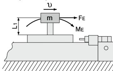
$$\therefore M_E = \frac{1}{3} \cdot F_E \cdot L_1 = 4.57\bar{v}a\delta m L_1 \text{ (N・m)}$$
